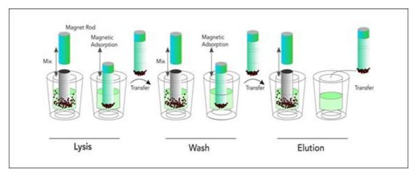
Figure 1-2. Principle steps of magnetic beads processing
